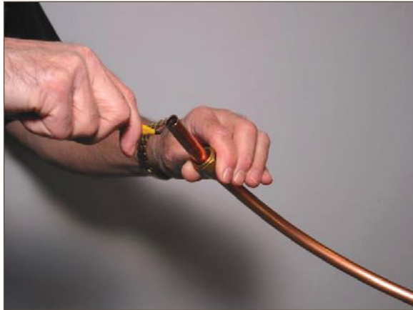
Figure 9.3. Reaming Prior to Flaring the Tube End
