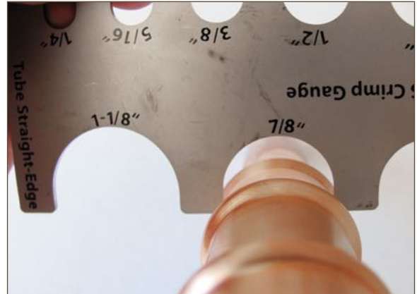
Figure 11.21. Un-crimped or improperly crimped fitting
