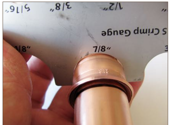
Figure 11.22. Correctly crimped fitting
