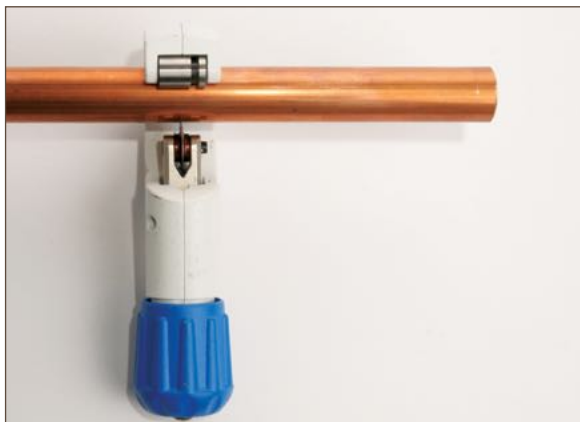
Figure 11.6. Cutting the tube square
