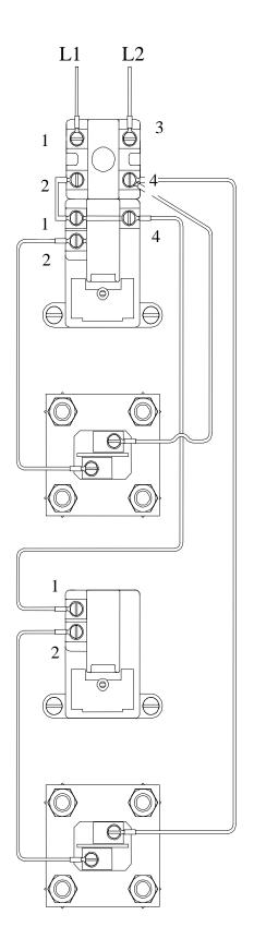
Interlocked for Non-Simultaneous Operation Operation
