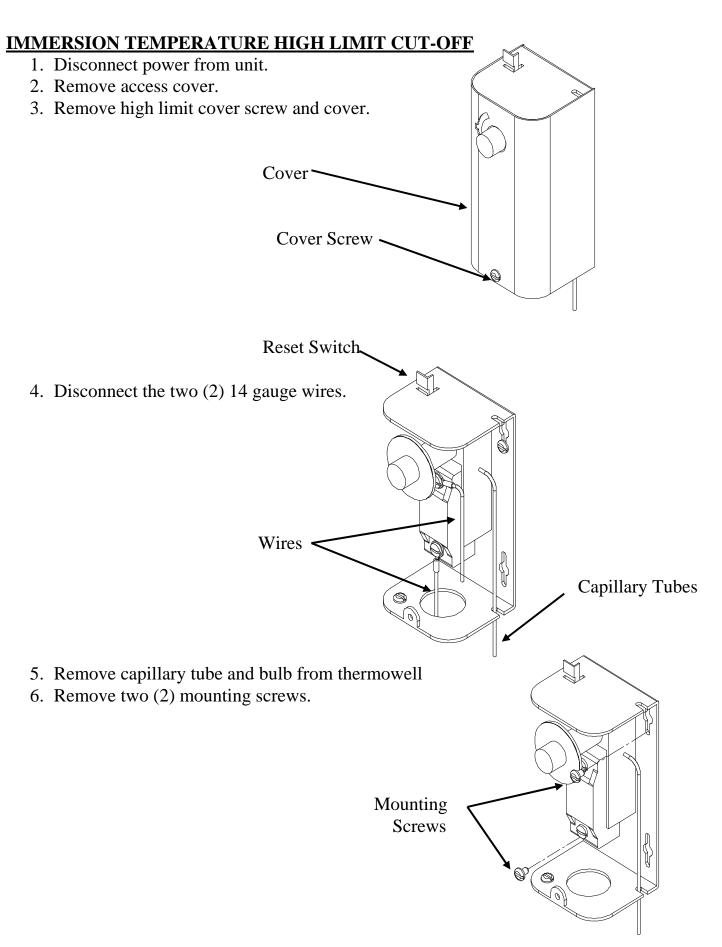
7. Remove control and install new high limit switch by performing above steps in reverse order. (Note: Be sure to place capillary tube into slot in base prior to installing cover.)
