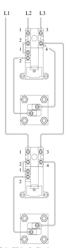
3 Ø Open Delta Wiring for Simultaneous Operation
