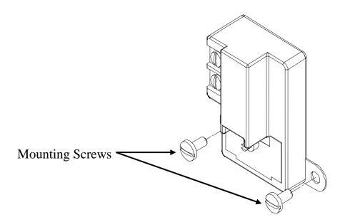
Replace thermostat using the reverse procedure.
