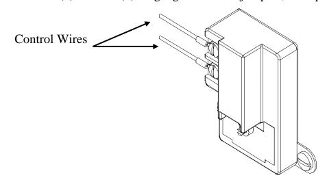
4. Remove two (2) mounting screws and disconnect from high limit cut-off, if required.
