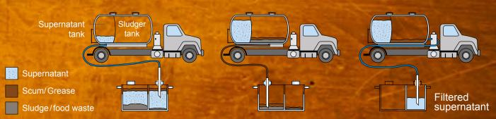
System detects density variations and automatically switches dispatchin of content from one tank to another.
