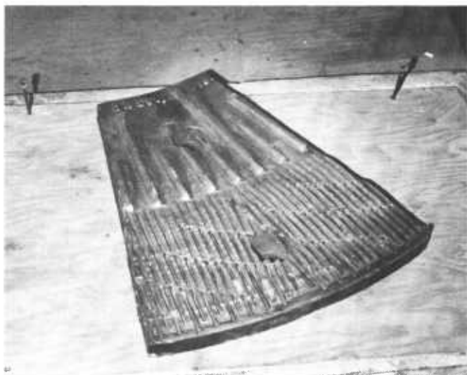
Figure 106 —Plate segment of Sprout-Waldron 42-in pressurized refiner.
