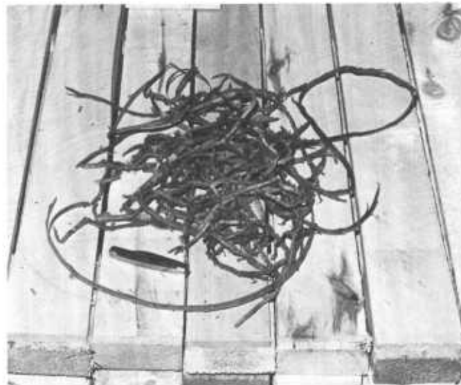
Figure 274 —Shavings generated by fixed panel-scoring knives.
