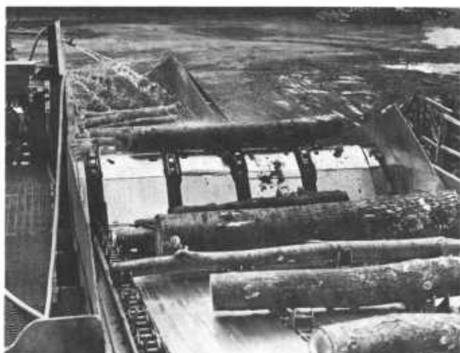
Figure 48 —Jack ladder. Water spray reduces friction, eases handling of logs.
