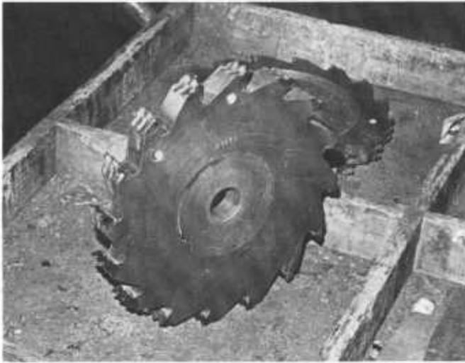
Figure 268 —Carbide-tipped cutterhead for rounding hardboard edges.
