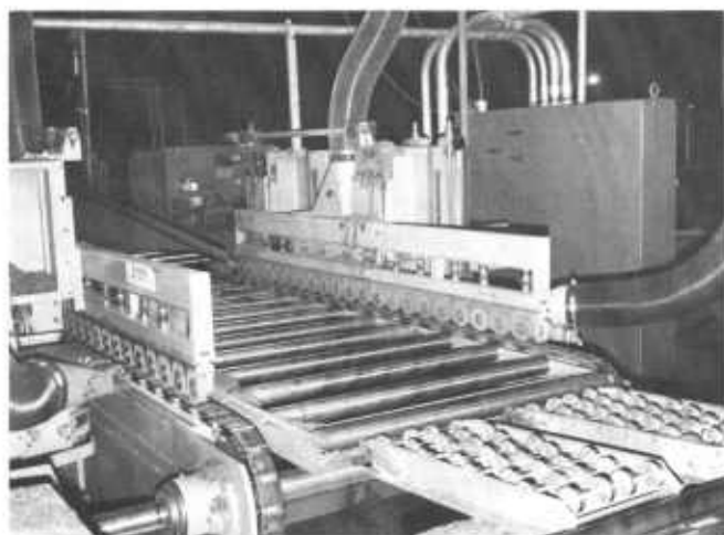
Figure 267 —Outfeed end of edge trimmer. Note feed chains and hold-down rolls.
