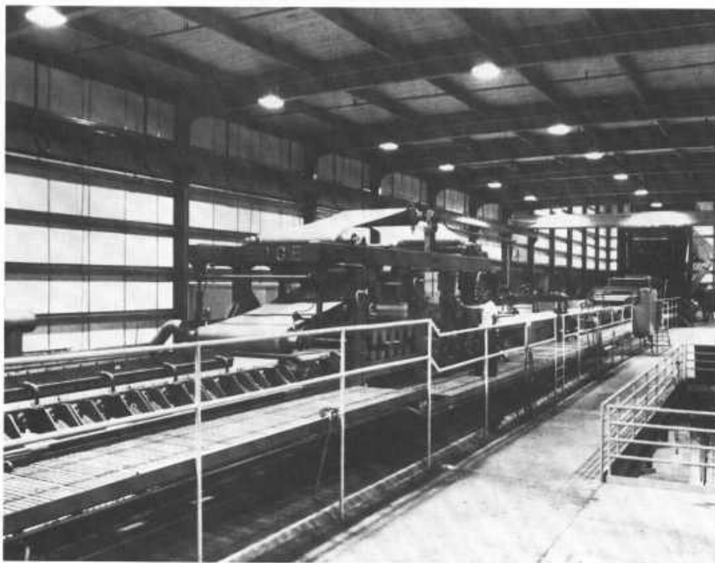
Figure 165 — Siempelkamp wet-process hardboard press line in western SIS fiberboard plant (Siempelkamp 1980).
