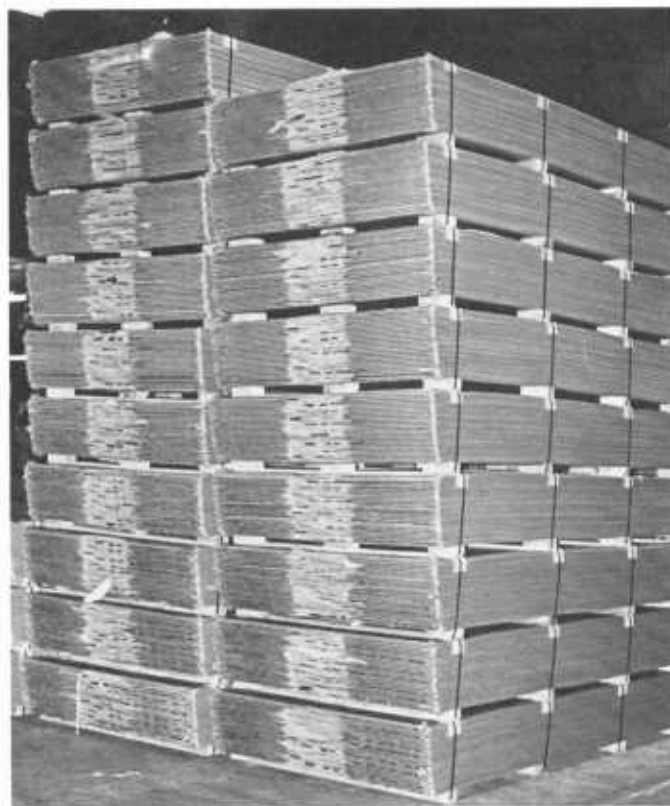
Figure 308 —Wrapped and unitized finished hardboard panels. Panels are wrapped individually. Spacer blocks and wood stringers are included in each package to facilitate handling by fork lift truck.
