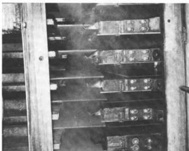
Figure 184 —Loading of S2S press. Mats are just entering press. Finished boards show some dislocation.
