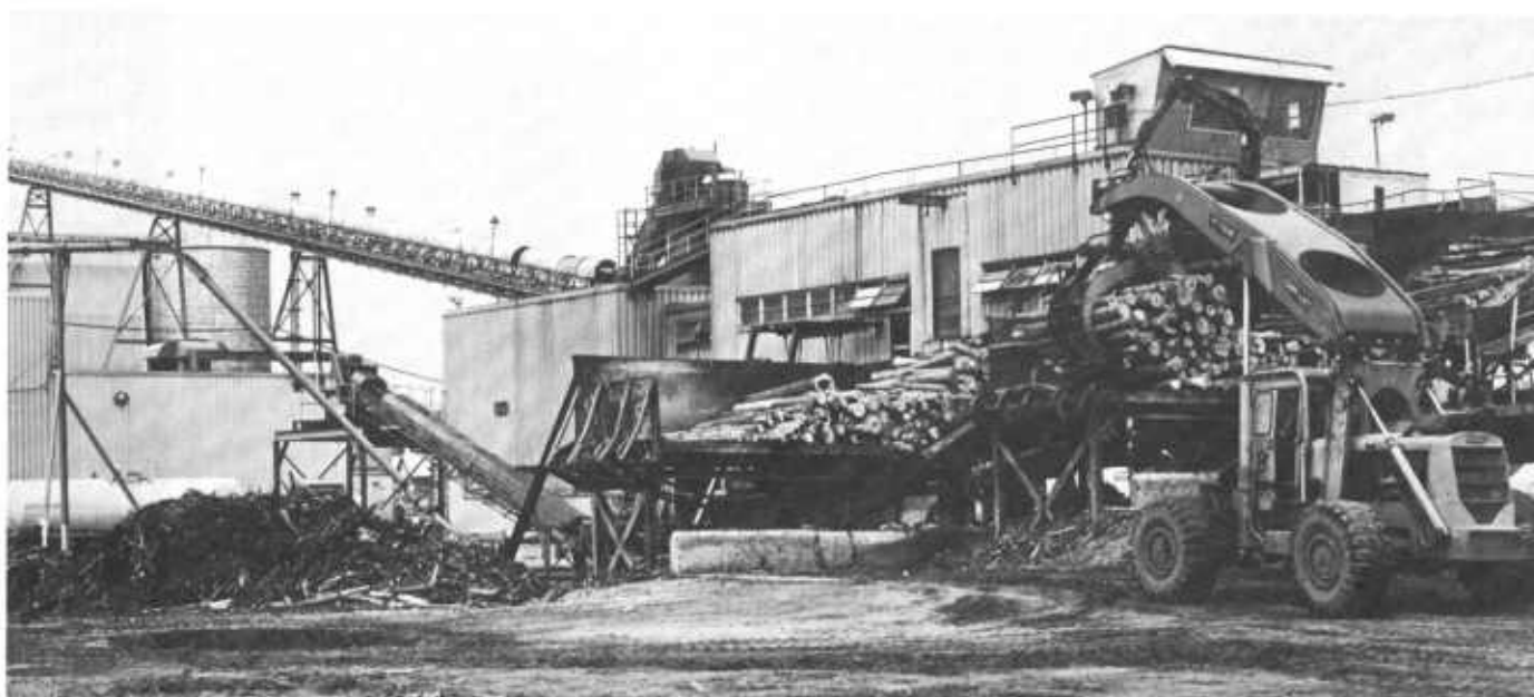
Figure 47 —Loading of roundwood on jack ladder for processing in woodroom. Belt conveyor in background delivers screened chips to silos.
