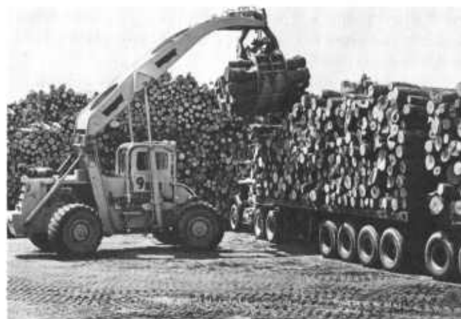
Figure 45—Unloading of truck in woodyard. Total load on truck and trailer approximately 14 cords.
