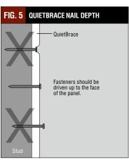
Fasteners should be placed no closer than  $\frac{3}{8}$ " from the edge and should be driven perpendicular to the face. Where two panels meet on a framing member, care must be taken in placing the fasteners so that both panels are fastened correctly on the common framing member.
