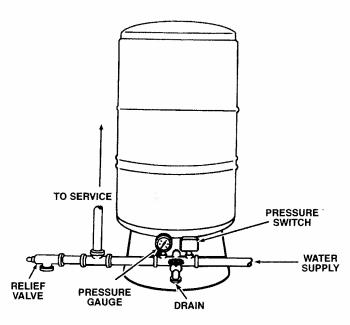
The water system tank should be installed as close as possible to the pressure switch (24 inches or less) to reduce the adverse effect of friction loss and elevation differences.
