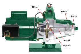
Centrifugal pumps, both the shallow-well and deep well types have little or no ability to pump air. When starting, the pump and suction line needs to have all of the air removed. An air leak in the suction line will cause the pump to quit pumping. This is or sometimes referred to as "losing its prime".
