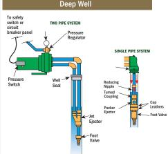
For a jet nozzle to be effective it must be combined with a venturi. The venturi changes the high-speed jet stream back to a high-pressure for delivery to the centrifugal pump. The jet and venturi are simple in appearance but they have to be well engineered and carefully matched to be efficient for various pumping conditions. The jet nozzle and venturi are also known as ejectors/ ejector kits.
