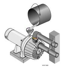
Figure 14 – Fill Pump Before Starting
