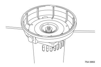
Figure 21 – Remove Seal plate
