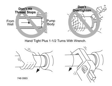
Figure 11 - Don't overtighten.
