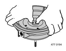
Figure 23 - Press in New Seal
