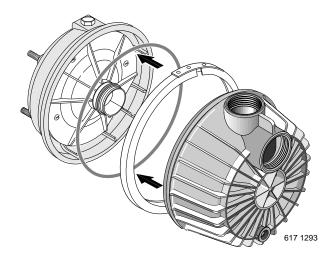
Figure 27 - Assemble Pump
