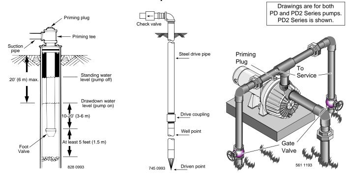
Figure 5 – Cased/Dug Well Installation
