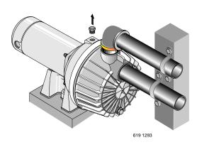
Figure 13 - Remove Priming Plug
