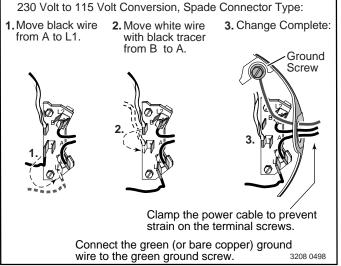
Figure 12 – 115/230V Dual Voltage Single Phase Wiring Diagram
