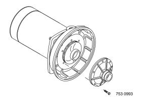
Figure 19 - Remove Diffuser
